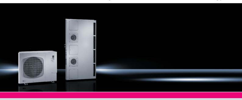
■ The cooling unit with inverter technology allows targeted speed control of the compressor. The coolant volume is regulated via the electronic expansion valve. Adaptation to cooling requirements facilitates energy savings of up to 40%. The cold air is expelled in front of the 482.6 mm (19″) level by the internal unit (evaporator coil), while the hot air is drawn in at the rear.
