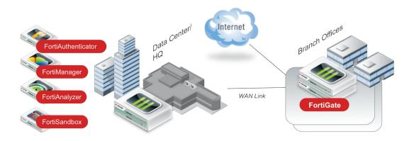
FortiGate deployed as branch office firewall
