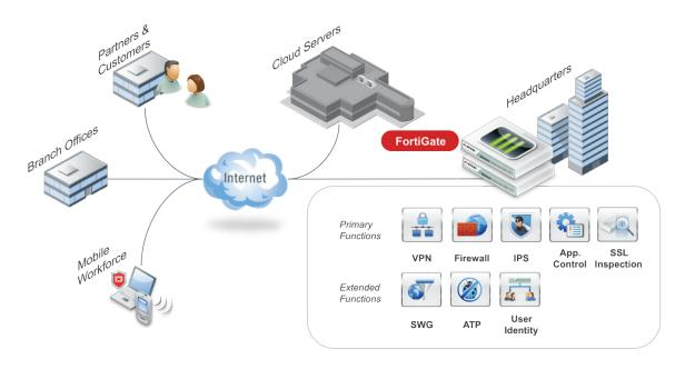
FortiGate deployed as mid enterprise edge firewall
