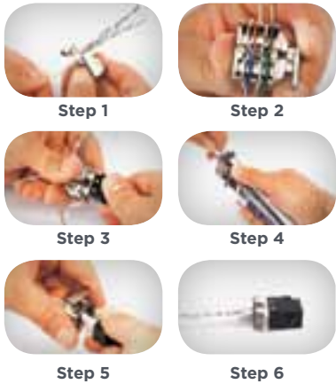
SL Series Modular Jack Termination Tool UTP Termination Method
